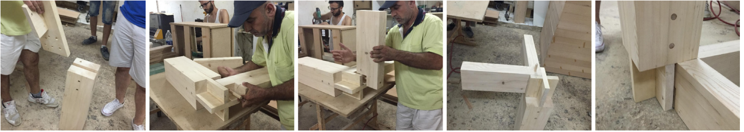
Figure 9: A full-scale prototype of the corner detail was mocked-up by a Syrian millworker who was eventually hired to do the wood work.
